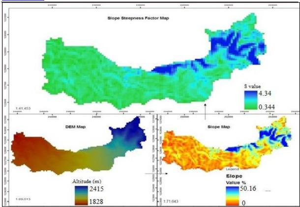
Figure 5: Derivation of steepness factor (S) from slope map
