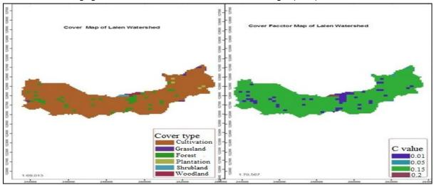
Figure 6: Derivation of cover factor from cover type
